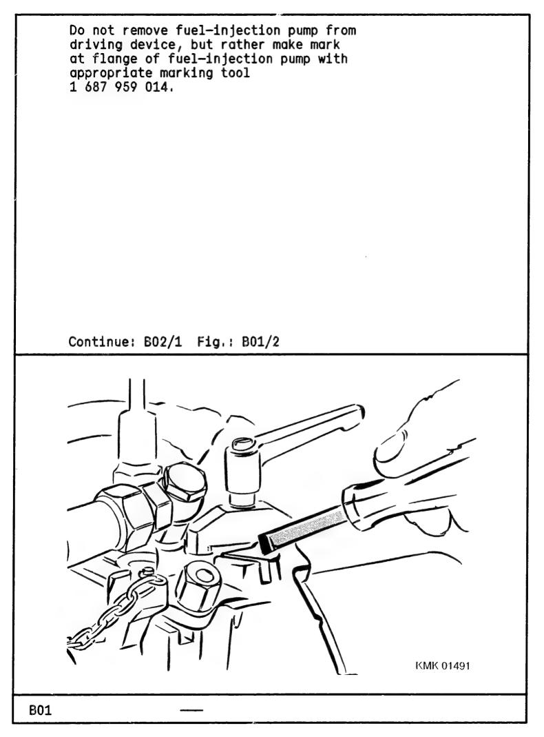
Move control rod to "O" position and set with setting mandrel of driving device.
